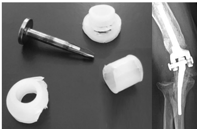
Fig. 3 Broken hinge of the Zimmer Coonrad – Morrey implant
