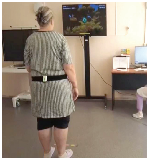
Fig. 1 An example of an inertial sensor installed during a patient examination and balance training using biofeedback
