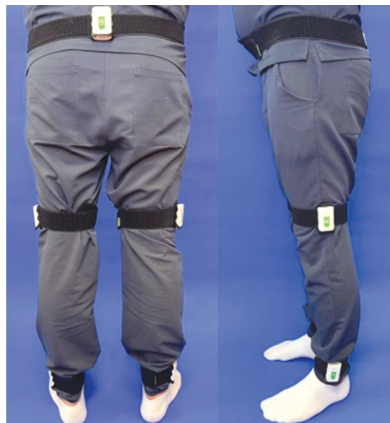
Fig. 1 An instance of inertial sensors placed for patient examination
