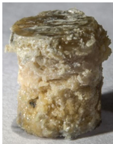
Fig. 3 The specimen upon completion of the mechanical test for uniaxial compression
