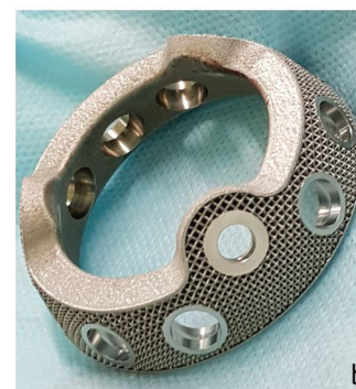
Fig. 2 Preoperative planning ( a ) and a customized implant ( b )
