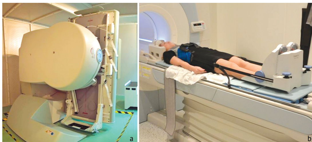
Fig. 1 MRI system with the possibility of verticalization (a); position of a patient during the study with a dosed axial load (b)
