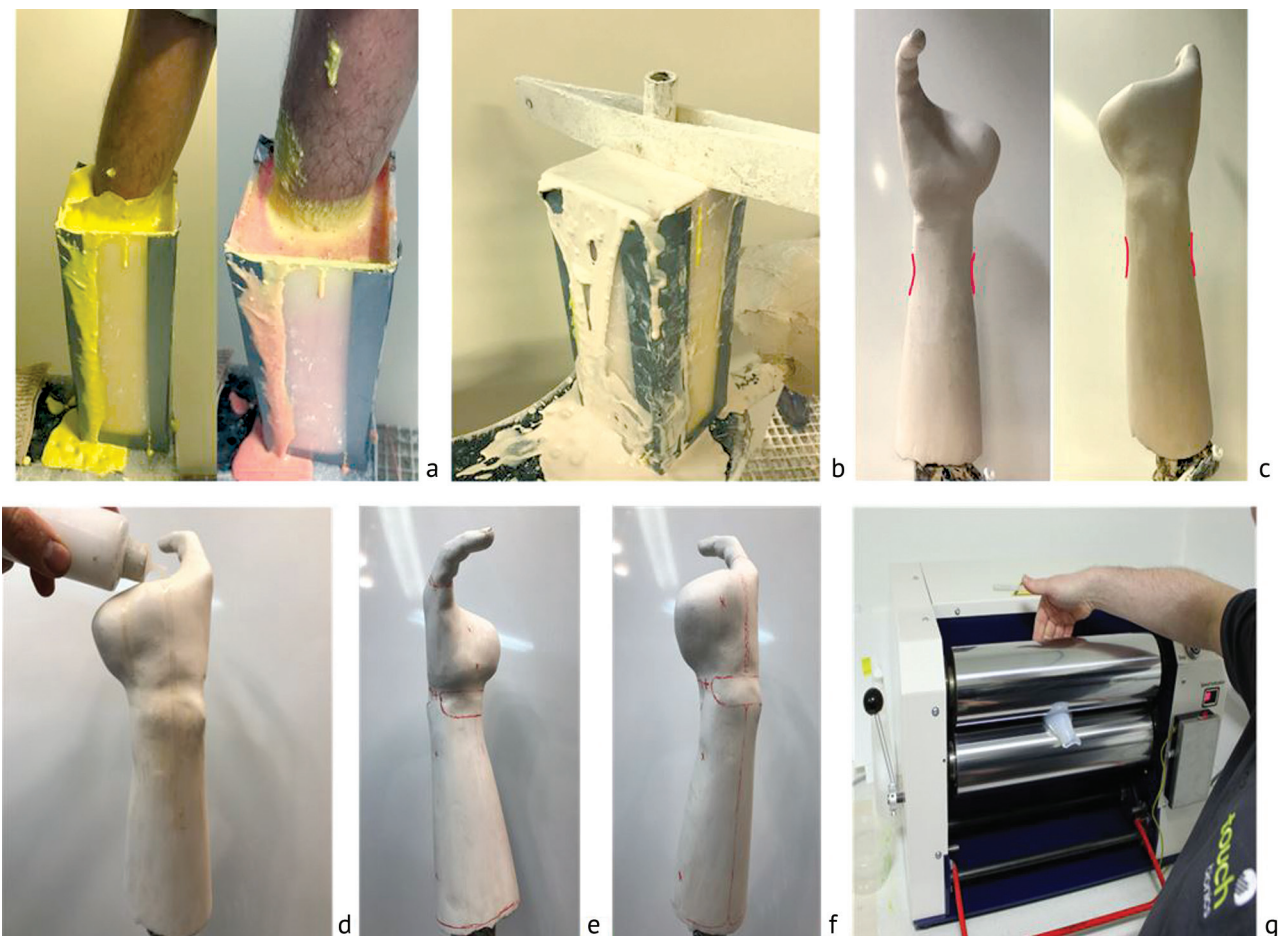
Fig. 1 Technological steps for production of a silicone socket for a functional prosthesis: a – damaged limb mold making with alginate; b – pouring liquid plaster into the alginate mold; c – processing of the positive plaster reproduction, drying; pelottes are marked red; d – application of a separating agent; e, f – marking of positive plaster reproduction; g – machine for mixing HTV silicone (rollers)
