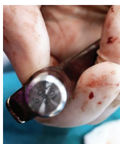
Fig. 1 Nonstandard cone of the femoral component
